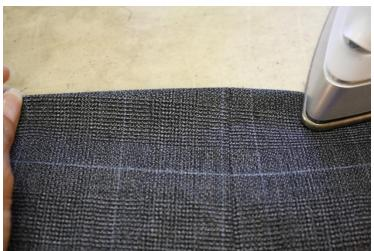
Press hem, using the front hem mark and the back hem mark as the guide.
