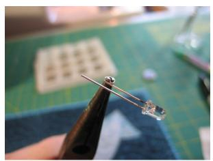
See how one leg of this LED is marked with the marker? That's the POSITIVE leg.
