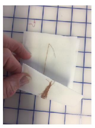
THUS.....if any machine is threaded with the presser foot DOWN, that the thread nest will likely result BECAUSE the thread cannot 'get seated' back in between the tension discs, therefore there is no 'squeeze' or 'tension' on it.
