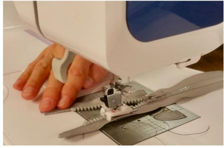
• Tie off the threads and use a bit of seam sealant to further secure the stitches. Remove excess zipper teeth above the bar tacks with an appropriate snipping tool, then fold tape back to finish or enclose excess zipper tape.
