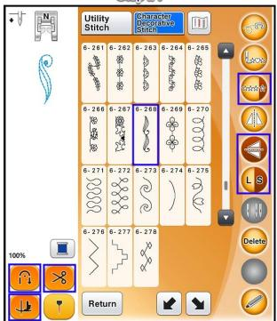
Select stitch 6-268, size small. Choose the single pattern option. Use horizontal flip option to turn the stitch. Activate tie off, pivot function, and auto cut features.
