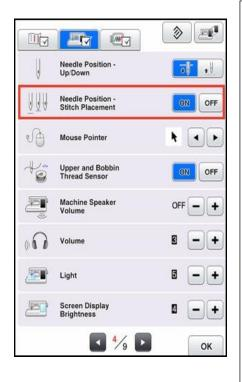
Select the option to "hover" over the fabric before stitching to help position individual stitches. This is called Needle Position Stitch Placement in the set mode.
