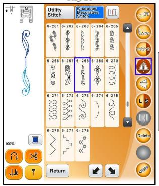
Select stitch 6-268. Choose the single pattern option. Deselect the horizontal flip option and mirror image the stitch to create stitch sequence shown here. Stitch this combination in the first thread color. **Tip**: Change to option for stitching a row if you want to stitch more than one segment of combined patterns.
